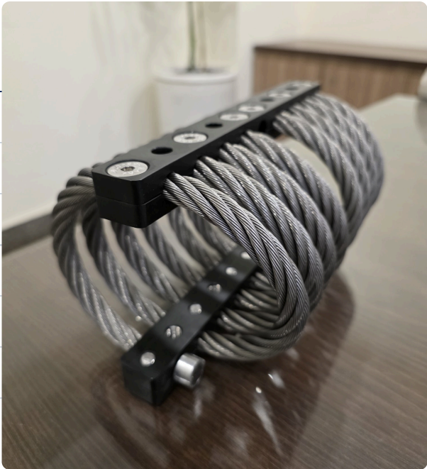
AWRI heavy isolator as supplied: stainless rope, black-finished retainer bars, stainless fasteners. All-metal, no ageing, works from -50 to +120 °C.
