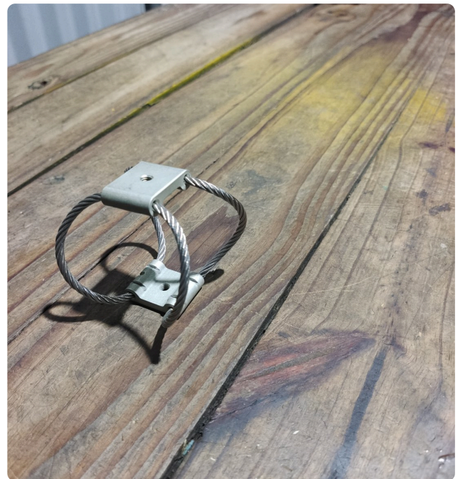
Compact isolator. Two-loop design with formed brackets, used for second-stage isolation of instruments inside an isolated shelter.
