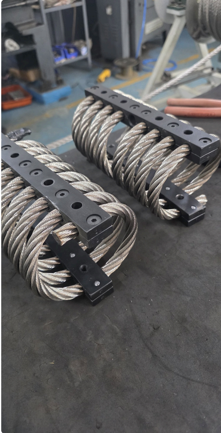
Heavy AWRI isolators on the assembly bench. Stainless rope, multi-loop winding, black-finished retainer bars clamped with socket-head screws. The heavy size class used in CargoRide packages.
